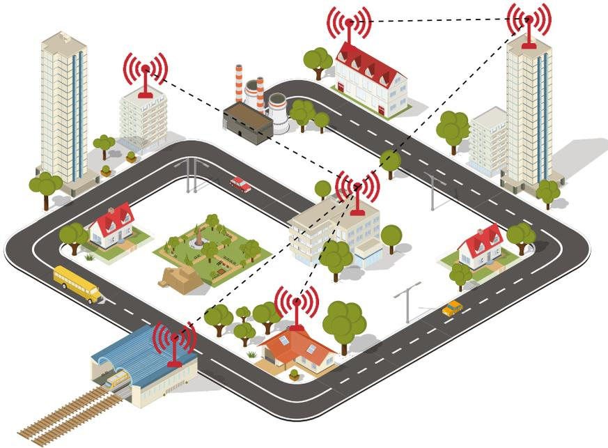
**EC SYSTEM** professional High Capacity point to multipoint microwave units allow radio data transmission up to 300 Mb throughput per sector. All models use MIMO technology with Adaptive Multipoint Access Protocol to improve the communication performance. The units have incorporated L2/L3 routers, allows GPS synchronization. Our base stations and subscriber terminal software gives to the customer the possibility of upgrade their networks adding transmission capability.
