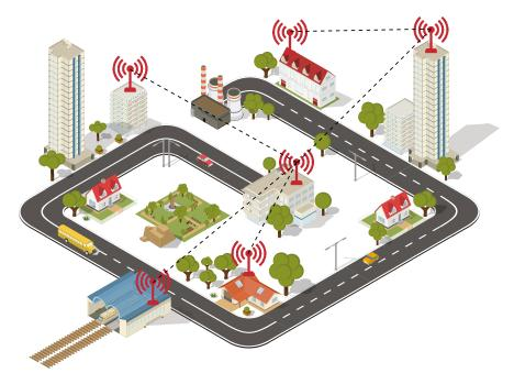
**EC LINK** is a Professional wireless Point-to-Point solution, which combines high-speed capability, up to 500 Mbps throughput and can achieve distances in excess of 80 Km. All models use MIMO technology to improve the communication performance. The units have incorporated L2/L3 routers and are fully compatible with our EC System multipoint solutions.
